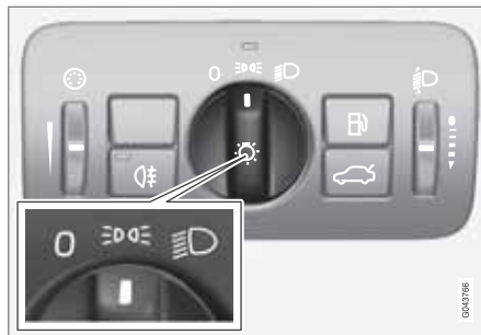
Headlamp control in position for position/parking lamps.
