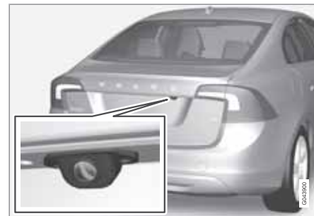
Camera location next to the opening handle.
