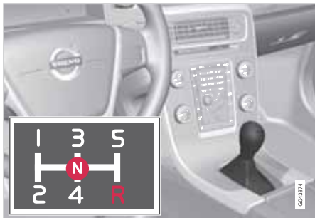
Gearshift pattern 5-speed gearbox.
