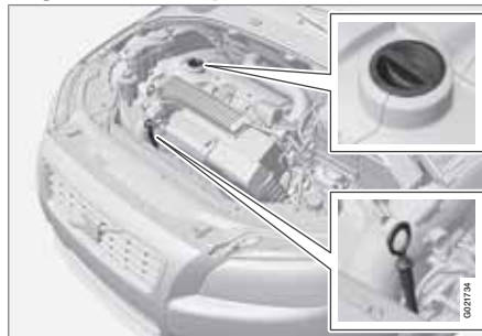
Dipstick and filler pipe.
