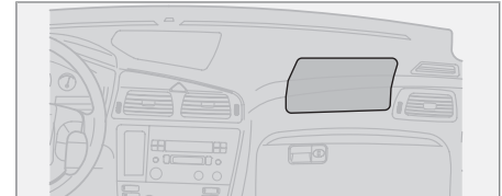
Location of the passenger airbag in left-hand drive and right-hand drive cars
