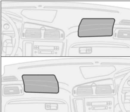
Location of the passenger airbag in left-hand drive and right-hand drive cars
