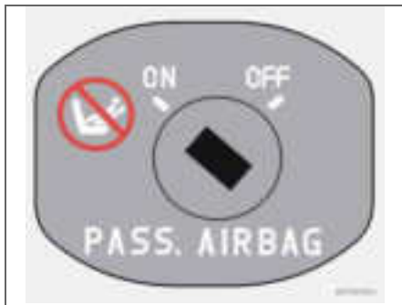
Switch for SRS in ON position.
