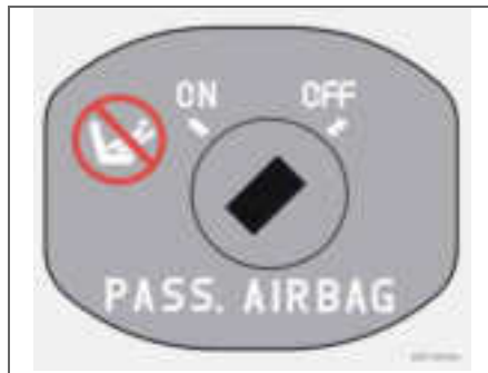
Switch for SRS in OFF position.
