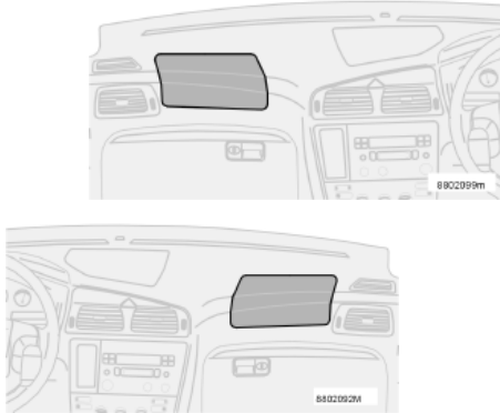
Location of the passenger airbag in left-hand drive and right-hand drive cars
