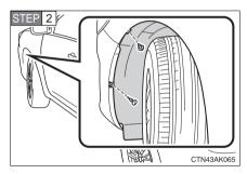
Remove the fender liner clips.
