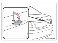
Turn the mechanical key clockwise to open.
