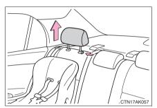
Remove the head restraint.
