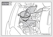
Add engine coolant if necessarv.
