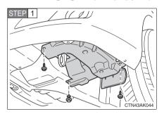
Remove the fender liner bolts and clip.
