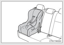
Seat belts equipped with a child restraint locking mechanism (ALR/ELR belts except driver's seat belt) (→P. 53)
