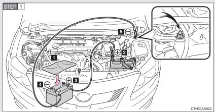
Connecting the jumper cables
