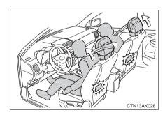
When a front seatback receives a strong impact, the head restraint moves slightly forward to help reduce the risk of whiplash on the seat occupant.
