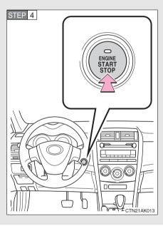
Press the "ENGINE START STOP" switch.
