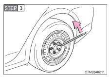
Slightly loosen the wheel nuts (one turn).
