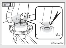
Before raising the vehicle, make sure that the floor jack is positioned so that the jack point fits securely inside the groove on the jack attachment.
