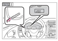
Press and hold the display button to enter the adjustment mode for the clock.
