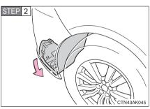
Partly remove the fender liner.
