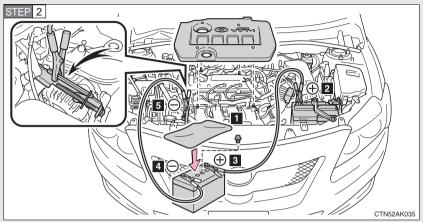
Connecting the jumper cables
