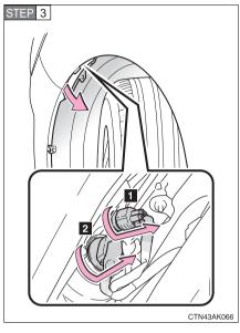
Partly remove the fender liner and turn the bulb base counter-clockwise.
