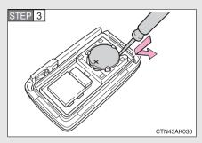
Remove the depleted battery.
