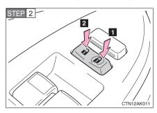
Shift the shift lever to P or N, and press and hold the driver's door lock switch (1 or 2) for approximately 5 seconds and then release.
