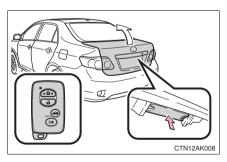
Press the button to unlock the trunk.
