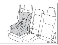
2 Latch the hook onto the anchor bracket and tighten the top tether strap.
