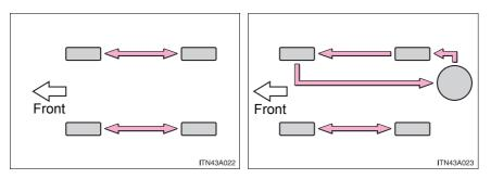
Do not fail to initialize the tire pressure warning system after tire rotation. To equalize tire wear and extend tire life, Toyota recommends that tire rotation is carried out at the same interval as tire inspection.
