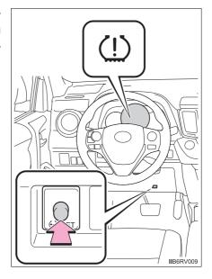
5 Vehicles without a smart key system: Wait for a few minutes with the engine switch in the "ON" position and then turn the engine switch to the "ACC" or "LOCK" position.
