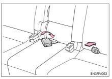
3 Lower the head restraint to the lowest position. ( $\rightarrow$ P. 146)
