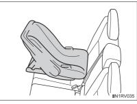
3 Run the seat belt through the child restraint system and insert the plate into the buckle. Make sure that the belt is not twisted.
