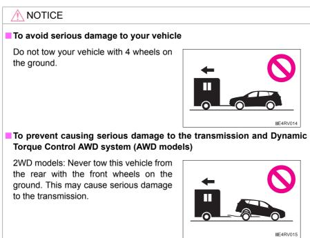
AWD models: Never tow this vehicle with any of the wheels on the ground. This may cause serious damage to the transmission and Dynamic Torque Control AWD system.
