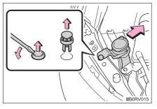
2 Disconnect the connector and turn the cover counterclockwise.
