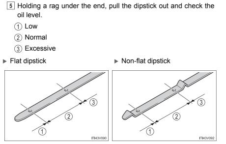
The shape of the dipstick may differ depending on the type of vehicle or engine.
