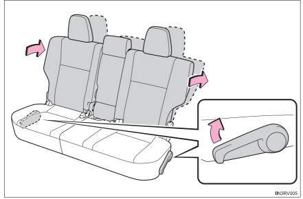
Pull up the lever. Then lean back to the desired angle and release the lever.
