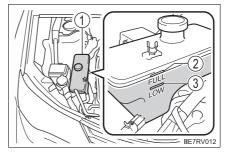
5 Add coolant if necessary. Water can be used in an emergency if coolant is unavailable.
