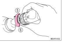
⑦ Washer/wiper dual operation The wipers will automatically operate a couple of times after the washer squirts.
