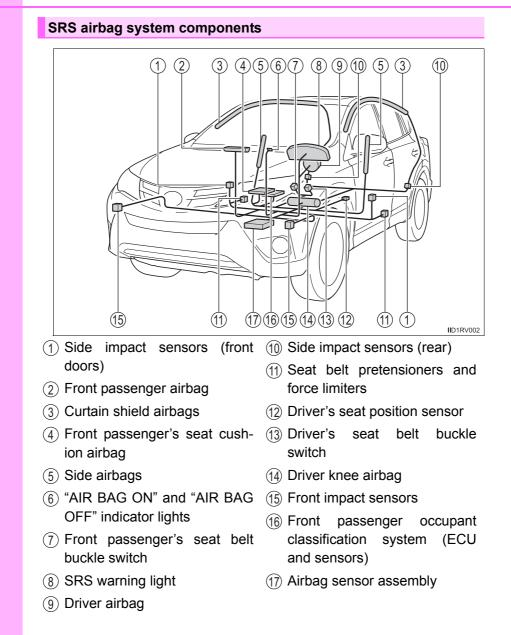
Your vehicle is equipped with ADVANCED AIRBAGS designed based on the US motor vehicle safety standards (FMVSS208). The airbag sensor assembly (ECU) controls airbag deployment based on information obtained from the sensors etc. shown in the system components diagram above. This information includes crash severity and occupant information. As the airbags deploy, a chemical reaction in the inflators quickly fills the airbags with non-toxic gas to help restrain the motion of the occupants.
