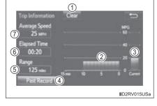
Average fuel consumption for the past 15 minutes is divided by color into past averages and averages attained since the engine switch was last turned to the "ON" position (vehicles without a smart key system) or IGNITION ON mode (vehicles with a smart key system). Use the displayed average fuel consumption as a reference.
