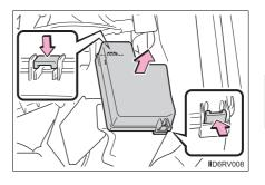
Under the instrument panel Remove the cover.
