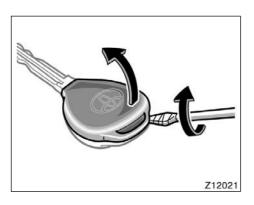
1. Open the cover using a flathead screwdriver wrapped with plastic tape.
