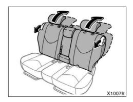
If the front hooks cannot be attached to the head restraint, push down the rear/second seatback.
