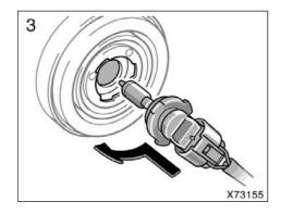
Pulg in a new bulb into the connector and install it into the mounting hole.
