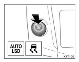
To turn on the system, push the "AUTO LSD" switch when the vehicle is stopped.
