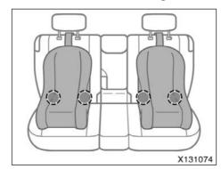
Lower anchorages for the child restraint systems complying with the FMVSS225 or CMVSS210.2 specifications are installed in the rear/second seat.
