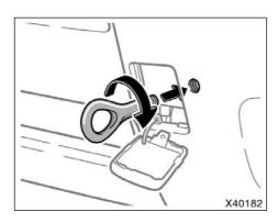
Use the front towing eyelet in the tool bag. Secure it to the hole on the bumper by turning clockwise. (For the tool bag location, see "—Required tools and spare tire" on page 356 in this Section.)
