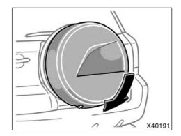
2. Attach the cover by hooking the 2 inner protrusions.
