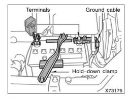
Check the battery for corroded or loose terminal connections, cracks, or loose hold-down clamp.
