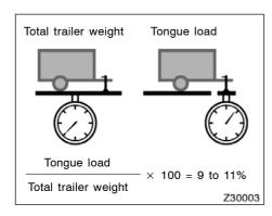
Never load the trailer with more weight in the back than in the front. About 60% of the trailer load should be in the front half of the trailer and the remaining 40% in the rear.
