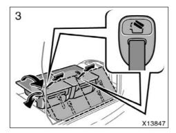
3. Pull and hold the seat lock release strap and lift up the seat rearward. Then push the seat down.
