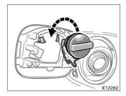
3. The removed cap can be hanged on the cap hanger.
