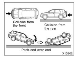
The curtain shield airbags are not generally designed to inflate if the vehicle is involved in a front or rear collision, if it pitches end over end, or if it is involved in a low-speed side collision.
