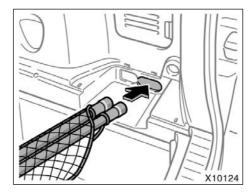
3. Insert the right end of the rear cargo net into the luggage storage box as shown.
