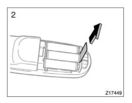
2. Remove the insulating sheet.
