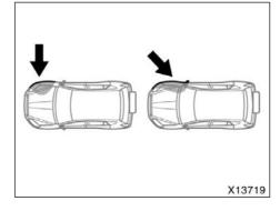
The curtain shield airbags may not activate if the vehicle is subjected to a collision from the side at certain angles, or a collision to the side of the vehicle body other than the passenger compartment as shown in the illustration.
