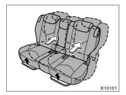
BEFORE USING LUGGAGE COVER Move the rear/second seats to the rearmost lock position.
