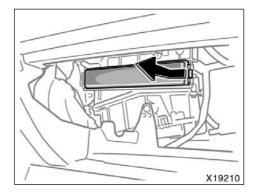
3. Remove the filter cover as shown in the illustration.
