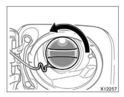
To remove the fuel tank cap, turn the cap counterclockwise. Pause slightly before removing it.
