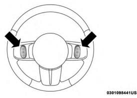
Remote Sound System Controls (Back View Of Steering Wheel)
