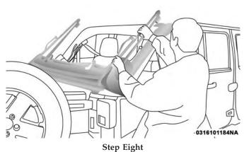
**NOTE:** Ensure the fabric does not overhang the sides of the vehicle.
