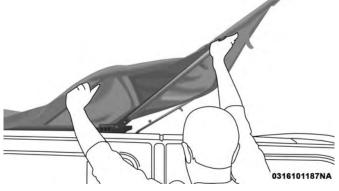
9. Open the header latches and engage the hook on each side onto the windshield loops (do not close the latches).
