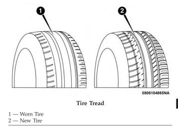
These indicators are molded into the bottom of the tread grooves. They will appear as bands when the tread depth becomes a 1/16 of an inch (1.6 mm). When the tread is worn to the tread wear indicators, the tire should be replaced. Refer to "Replacement Tires" in this section for further information.
