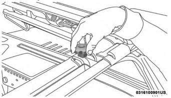
Step Five Door Frame Installation — Four Door Models — If Equipped 2. Set the door frame pin into the hole on top of the body side, just behind the rear door opening.
