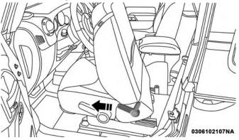
Rotate the entire seat assembly toward the instrument panel.
