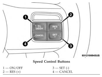
**NOTE:** In order to ensure proper operation, the Speed Control System has been designed to shut down if multiple Speed Control functions are operated at the same time. If this occurs, the Speed Control System can be reactivated by pushing the Speed Control ON/OFF button and resetting the desired vehicle set speed.
