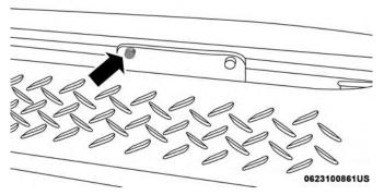
**Bodyside Nut** 2. Remove one bolt from the underside of the vehicle.
