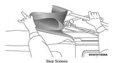
17. Fold the top so that the material forms a "W" as shown. Enter the vehicle and move the material into two folds.
