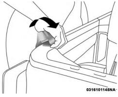
15. Completely release the latches from the loops on the windshield frame. If your vehicle is not equipped with the Sunrider package, proceed to Step 18.
