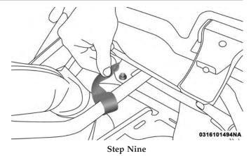
10. Remove the swing gate bar (black metal bar for bottom of rear window) and set aside.
