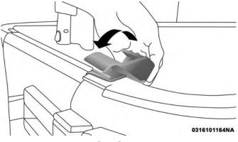
8. Move to the rear of the vehicle and gently pull the sail panels over the rear roof bow.
