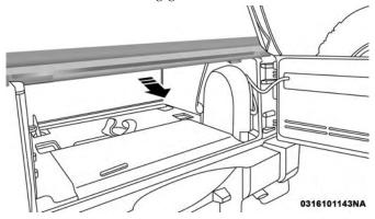
6. Unzip the rear window starting at the right lower corner of the window. Pull the zipper up, across the top and down to the left lower corner. **Zipper pulls will stay on the rear window.** Pull down on the rear window to disengage it from the zipper on the top cover.
