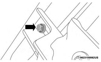
**Underside Bolt** 3. Remove the side step assembly.
