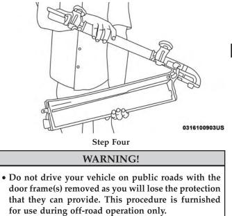
• Do not drive your vehicle on public roads with the doors removed as you will lose the protection that they can provide. This procedure is furnished for use during off-road operation only.
