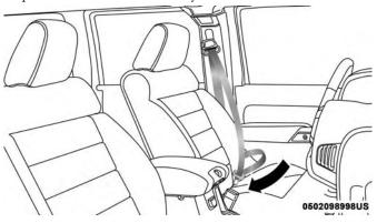
Inserting Latch Plate Into Buckle
