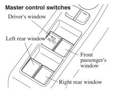
To open the window to the desired position, hold down the switch. To close the window to the desired position, pull up the switch.
