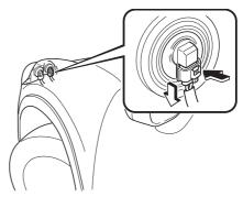
5. Turn the socket and bulb assembly to remove it. Carefully remove the bulb from its socket in the reflector by gently pulling it straight backward out of the socket.
