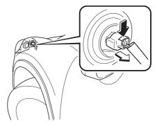
4. Turn the socket and bulb assembly to remove it. Carefully remove the bulb from its socket in the reflector by gently pulling it straight back out of the socket.
