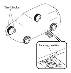
Use only the front and rear jacking positions recommended in this manual:
