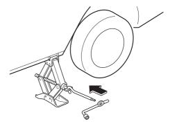
8. Turn the jack handle clockwise and raise the vehicle high enough so that the spare tire can be installed. Before removing the lug nuts, make sure your Mazda is firmly in position and that it cannot slip or move.
