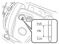
Pull it out again and examine the level. The level is normal if it is between Low and Full.
