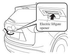
When the ignition is switched ON: The liftgate can be opened only when the vehicle is stopped with the parking brake applied (manual transaxle), or with the shift lever in the P position (automatic transaxle).
