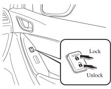
To lock all the doors/liftgate from an open front door, press the lock side of the door lock switch and then close the door.
