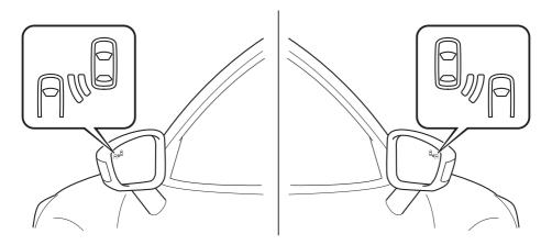
This warning light illuminates for a few seconds when the ignition is switched ON. If the BSM system detects a vehicle in the detection area while the vehicle is driven at a speed of about 32 km/h (20 mph) or more, the BSM warning light illuminates on the side of the vehicle where the rear on-coming vehicle is detected.
