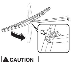
To prevent damage to the rear window, do not let the wiper arm fall on it. 3. Pull down the blade rubber and slide it out of the blade holder.
