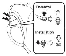
4. Turn the screw counterclockwise and remove it, and then partially peel back the mudguard.
