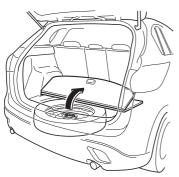
2. Secure the trunk board by attaching the hook to the head restraint.
