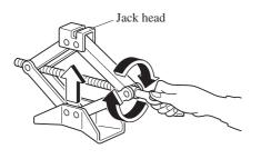
5. Place the jack under the jack-up position closest to the tire being changed with the jack head squarely under the jack-up point.
