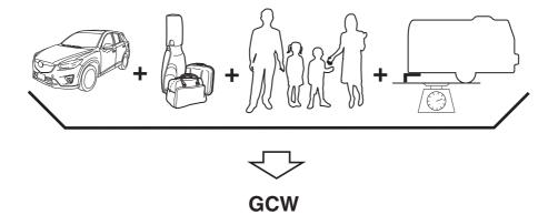
**GCW (Gross Combination Weight)** is the weight of the loaded vehicle (GVW) plus the weight of the fully loaded trailer.
