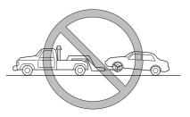
Do not tow the vehicle pointed backward with driving wheels on the ground. This may cause internal damage to the transaxle.
