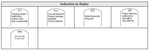
Action: Consult an Authorized Mazda Dealer to have your vehicle inspected. View the symbol indicated in the upper part of the screen and refer to the "Indication and method for taking action list" containing the symbol to see what action should be taken.
