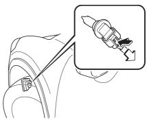
6. Turn the socket and bulb assembly to remove it. Carefully remove the bulb from its socket in the reflector by gently pulling it straight back out of the socket.
