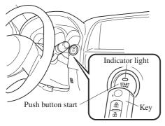
4. After the push button start indicator light (green) changes to full illumination, press the push button start with your finger.
