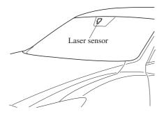
Always keep the surface of the windshield around the laser sensor clean to assure proper operation of the Smart City Brake Support (SCBS) system.
