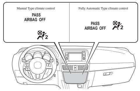
If the front passenger weight sensors are normal, the indicator light illuminates when the ignition is switched ON. The light turns off after a few seconds. The front/passenger air bag deactivation indicator light illuminates or is off under the following conditions:
