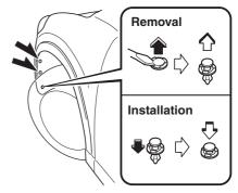
4. Turn the screw counterclockwise and remove it, and then partially peel back the mudguard.
