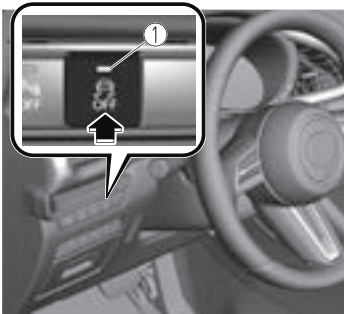
1. DSC OFF switch indicator light
