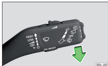
Fig. 189 Setting the service position for the wiper arms
