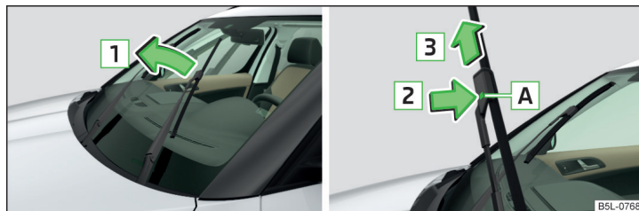
Fig. 190 Changing the windscreen wiper blade
