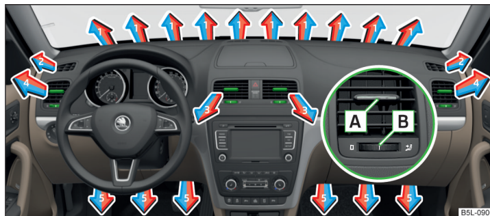
Fig. 117 Air vents at the front
