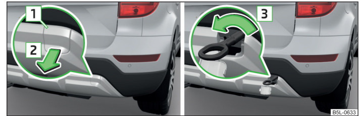
Fig. 182 Removing the cap / installing the towing eye
