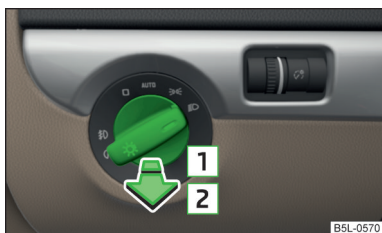
Fig. 28 Light switch: Switch on the front fog lamp
