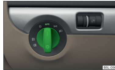
Fig. 27 Light switch: AUTO position
