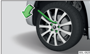
Fig. 174 Changing a wheel: Loosening the wheel bolts
