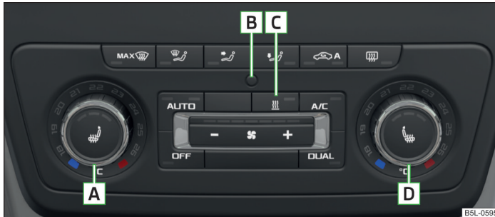
Fig. 95 Climatronic: Control elements
