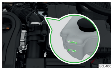
Fig. 162 Engine compartment: Brake fluid reservoir
