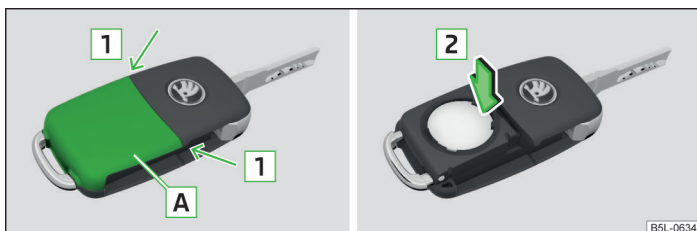
Fig. 183 Remove cover/take out battery
