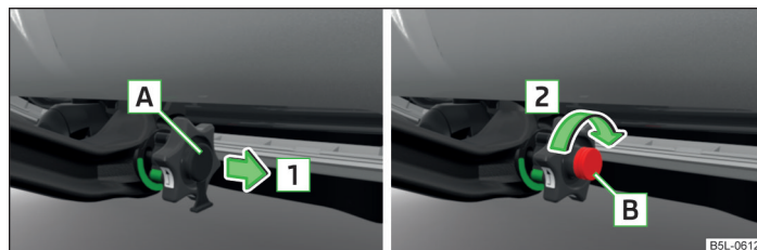
Fig. 132 Removing the lock cover/releasing the lock
