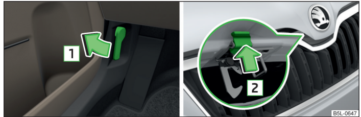
Fig. 156 Bonnet release lever/release lever
