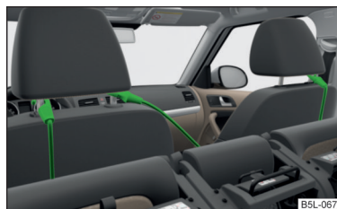
Fig. 50 Safety position of seat belt / folding the seat completely forward
