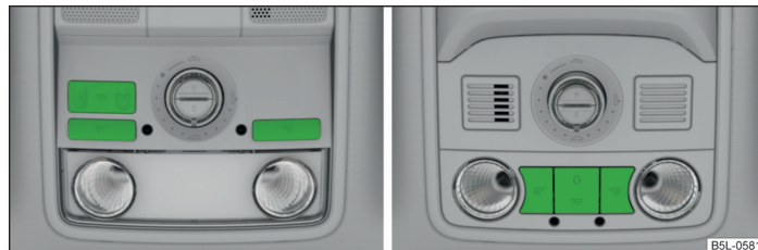
Fig. 31 Operation of the front interior light: Version 1/version 2
