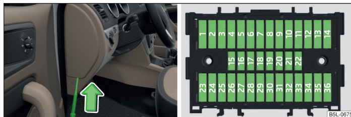
Fig. 193 Cover of the fuse box in the control panel / fuses
