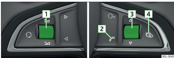
Fig. 98 Multifunction steering wheel: Control buttons for the telephone
