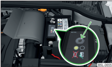
Fig. 164 Vehicle battery: Electrolyte level indicator
