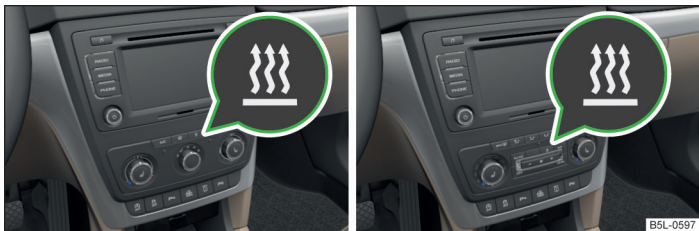
Fig. 96 Button for switching on/off the system directly on the operating part of the air conditioning/Climatronic
