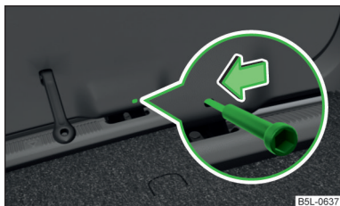
Fig. 188 Emergency unlocking of the boot lid
