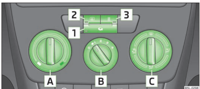
Fig. 88 Heating: Control elements
