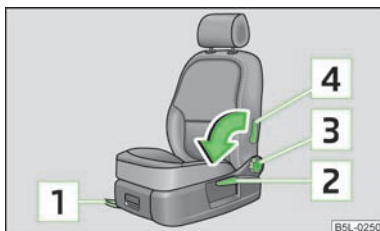
Fig. 41 Control elements at the seat
