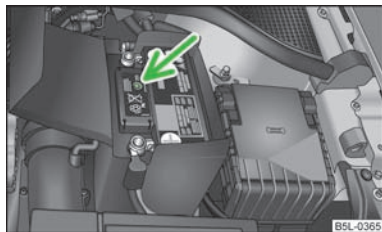
Fig. 149 Vehicle battery: Electrolyte level indicator
