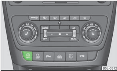
Fig. 105 Button for the START-STOP system
