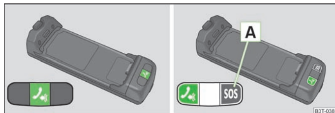
Fig. 111 Principle sketch: single-button adapter/two-button adapter
