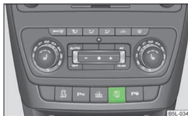
Fig. 155 Button for setting the tyre inflation pressure control value
