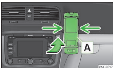
Fig. 110 Universal telephone preinstallation
