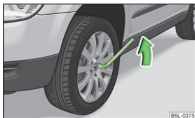
Fig. 158 Changing a wheel: Slackening wheel bolts
