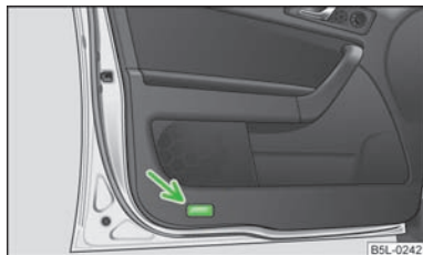
Fig. 33 Front door: Warning light
