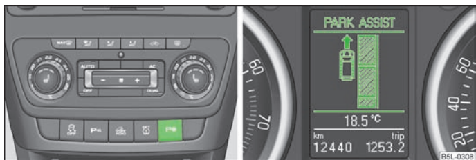
Fig. 101 Switch on display of the park assist in the information display/information display: Finding a suitable parking space
