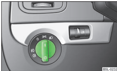
Fig. 23 Dash panel: Light switch
