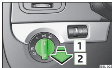
Fig. 25 Dash panel: Light switch
