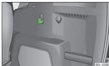
Fig. 55 Luggage compartment: folding hooks
