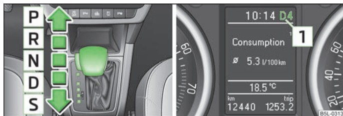
Fig. 106 Selector lever/information display: Selector lever positions
