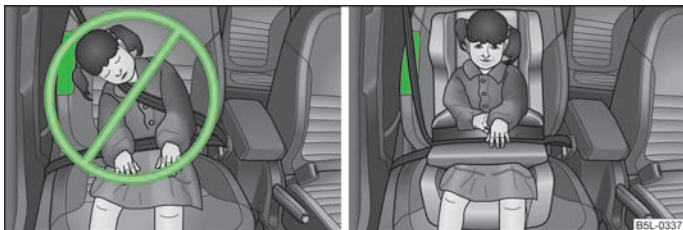
Fig. 130 Incorrect seated position of a child who is not properly secured - risk from side the airbag/Child properly protected by safety seat
