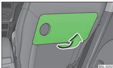
Fig. 79 Folding table on the front seat rest
