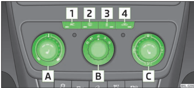
Fig. 89 The air conditioning system: Control elements
