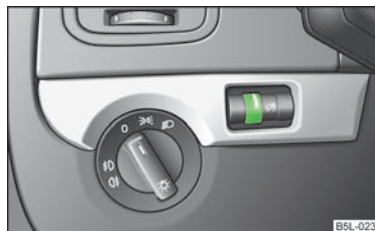
Fig. 26 Dash panel: Instrument lighting
