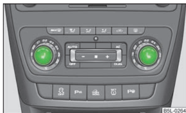
Fig. 45 Dash panel: Control for heating the front seats
