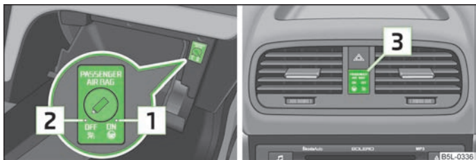
Fig. 129 Storage compartment: Switch for the front passenger airbag/indicator light for the deactivated front seat passenger airbag
