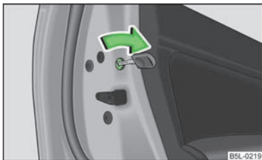
Fig. 10 Child safety locks on the rear doors
