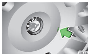
Fig. 154 Pull off the wheel trim cap on light alloy wheels
