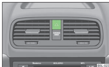
Fig. 28 Dash panel: Switch for hazard warning lights
