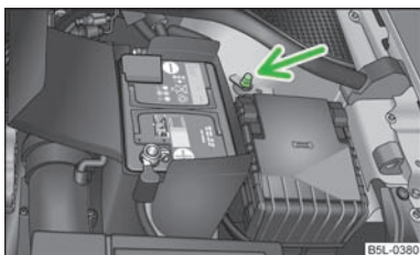
Fig. 164 Jump-starting - START-STOP system
