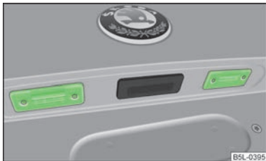
Fig. 175 Luggage compartment door Licence plate light
