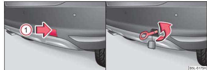
Fig. 183 Rear bumper: Removing the cover / installing the towing eye
