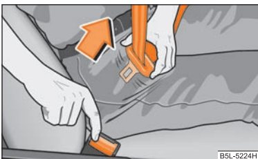
Fig. 128 Releasing lock tongue from belt lock
