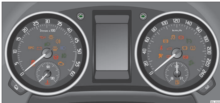
Fig. 21 Instrument cluster with warning lights
