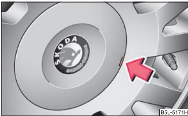
Fig. 177 Pulling off wheel trim cap on light alloy wheels
