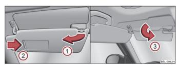
Fig. 56 Sun visor: Swivelling out / double sun visor: Folding out
