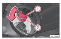
Fig. 202 Remove the bulb for daylight driving lights
