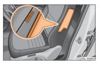
Fig. 141 Installation position of side airbag in driver seat
