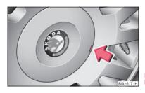
Fig. 185 Pulling off wheel trim cap on light alloy wheels
