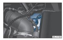
Fig. 174 Engine compartment: Brake fluid reservoir
