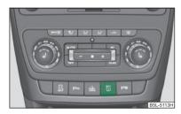
Fig. 156 Button for setting the tyre inflation pressure control value
