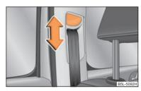
Fig. 135 Front seat: Seat belt height adjuster
