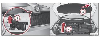
Fig. 13 Radiator grille: Locking lever / securing the bonnet with the bonnet support
