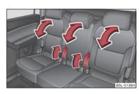
Fig. 68 Adjusting the seat backrest
