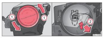
Fig. 198 Remove cap / removing the fixture for the parking light (halogen headlight)
