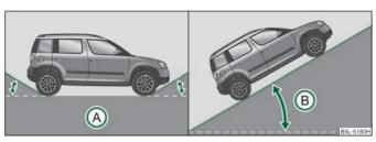
Fig. 163 Embankment angle / slope angle
