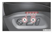
Fig. 64 Driver seat: Memory buttons and SET button
