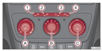
Fig. 109 Climatic: Control elements
