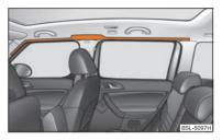
Fig. 143 Installation position of the head airbags
