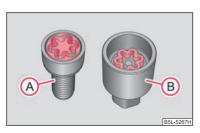
Fig. 188 Safety wheel bolt with adapter
