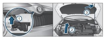
Fig. 170 Radiator grille: Locking lever / securing the bonnet with the bonnet support
