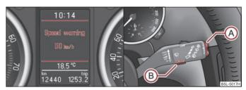
Fig. 21 Warning against excessive speeds / multi-functional indicator: Control elements
