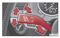
Fig. 50 Turn signal and main beam lever
