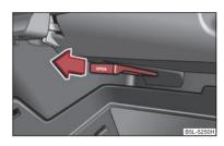
Fig. 95 Storage compartment: Using cooling system
