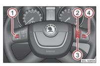
Fig. 128 Multifunction steering wheel: Control buttons for the telephone
