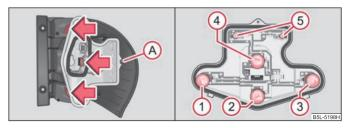
$Fig.\ 204\ \ Remove\ the\ middle\ part\ of\ the\ light\ /\ rear\ light\ unit:\ Fitting\ position\ of\ the\ bulbs$
