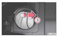
Fig. 199 Removing the fixture for the parking light (Xenon headlight)
