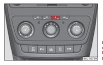
Fig. 111 Button for direct switching on/off of the auxiliary heating (auxiliary heating and ventilation) on the operating part of the Climatic
