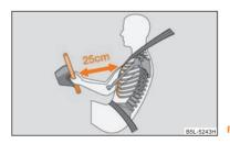
Fig. 139 Safe distance to steering wheel
