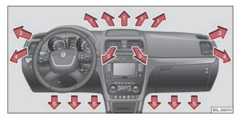
Fig. 106 Air vents at the front
