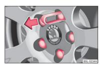
Fig. 184 Removing the cap
