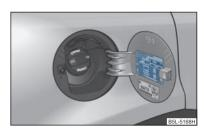
Fig. 178 An opened fuel filler flap with a tyre size and tyre inflation pressure table
