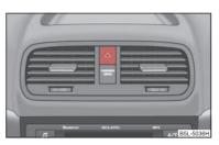
Fig. 49 Dash panel: Switch for hazard warning lights
