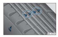
Fig. 179 Tyre tread with wear indicators
