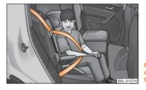
Fig. 150 Child seat in Group 2 installed on the rear seat facing the direction of travel
