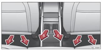
Fig. 107 Air vents at the rear
