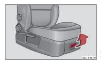
Fig. 100 Front passenger seat: Storage compartment
