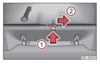
Fig. 37 Emergency unlocking of the boot
