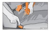
Fig. 136 Releasing lock tongue from belt lock
