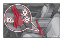
Fig. 105 Securing the removeable through-loading bag
