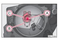
Fig. 200 Removing the bulb for the main beam light and low beam light
