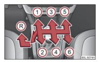
Fig. 115 The shift pattern: 5-speed or 6speed manual gearbox
