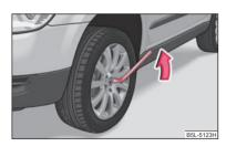
Fig. 186 Changing a wheel: Slackening wheel bolts
