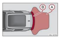
Fig. 117 Parking aid: Detection range of rear sensors
