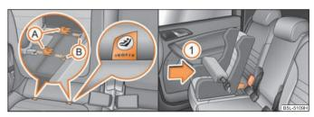
Fig. 152 Locking eyes (ISOFIX system) / the ISOFIX child seat is pushed into the mounting funnels
