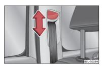
Fig. 4 Front seat: Seat belt height adjuster
