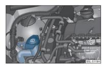
Fig. 177 Engine compartment: Windshield washer fluid reservoir
