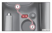
Fig. 34 Centre console: Buttons for central locking
