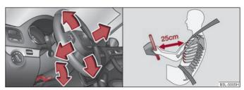
Fig. 3 Adjustable steering wheel: Lever on the steering column / the correct distance of the driver from the steering wheel
