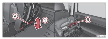
Fig. 70 Unlocking the folded forward seat / carrying handles on the seat cushion
