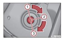
Fig. 114 Ignition lock positions
