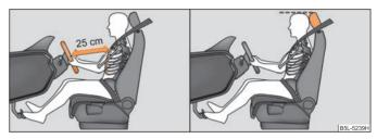
Fig. 131 The correct distance of the driver from the steering wheel / the correct head restraint adjustment for the driver
