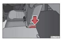
Fig. 72 Folding the seat backrest back into position
