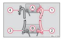
Fig. 189 Jump-starting using the battery from another vehicle: A - flat vehicle battery. B - battery providing current
