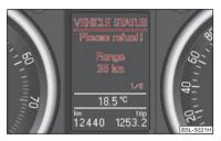
Fig. 25 Information display: Display of operational fault
