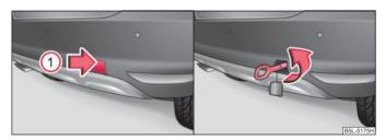
Fig. 191 Rear bumper: Removing the cover / installing the towing eye
