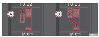
Fig. 120 Information display: the determined parking space with the information to drive on (A) and for engaging the reverse gear (B)
