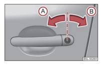
Fig. 33 Turning the key for unlocking and locking the vehicle
