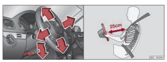
Fig. 113 Adjustable steering wheel: Lever below steering column / safe distance to steering wheel
