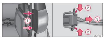
Fig. 203 Removing the rear light unit / disconnecting the plug connection
