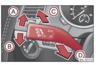
Fig. 8 Turn signal and main beam lever
