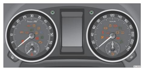
Fig. 29 Instrument cluster with warning lights
