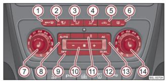
Fig. 110 Climatronic: Control elements
