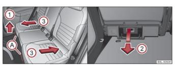
Fig. 67 Releasing at the front / rear
