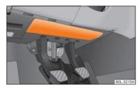
Fig. 140 Driver's knee airbag below the steering column
