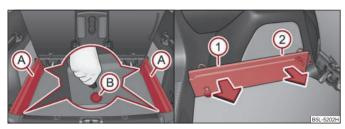
Fig. 82 Luggage compartment: Slacken check points / remove carrier rails
