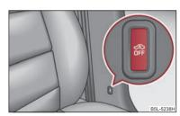
Fig. 39 Button for interior monitor and towing protection monitoring
