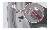
Fig. 35 Rear door: Emergency locking of the door
