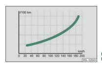
Fig. 160 Fuel consumption in litres/100 km. and speed in km/h.
