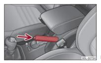
Fig. 116 Centre console: Handbrake
